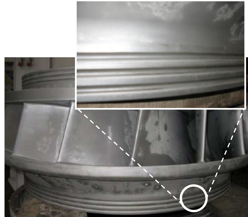
Runner coated with tungsten carbide after facing 159.000 t Sediment: without damages
